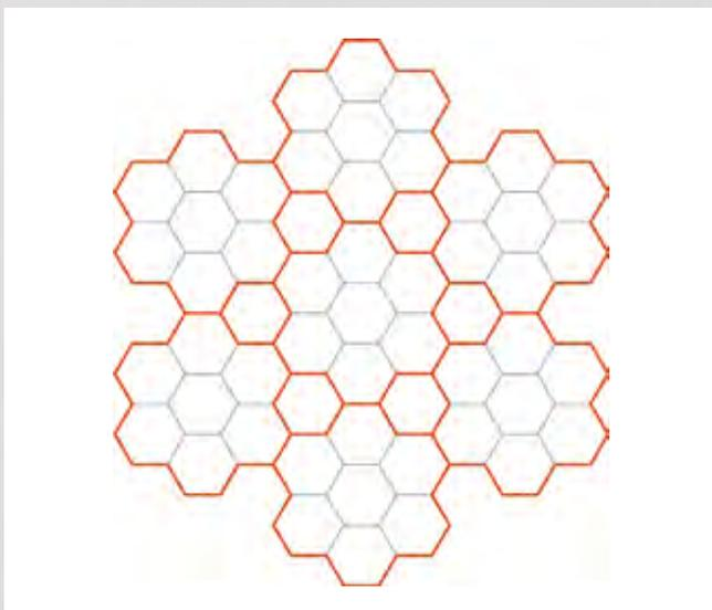
The diagram below shows the construction of the 7 x 19 wire braids
