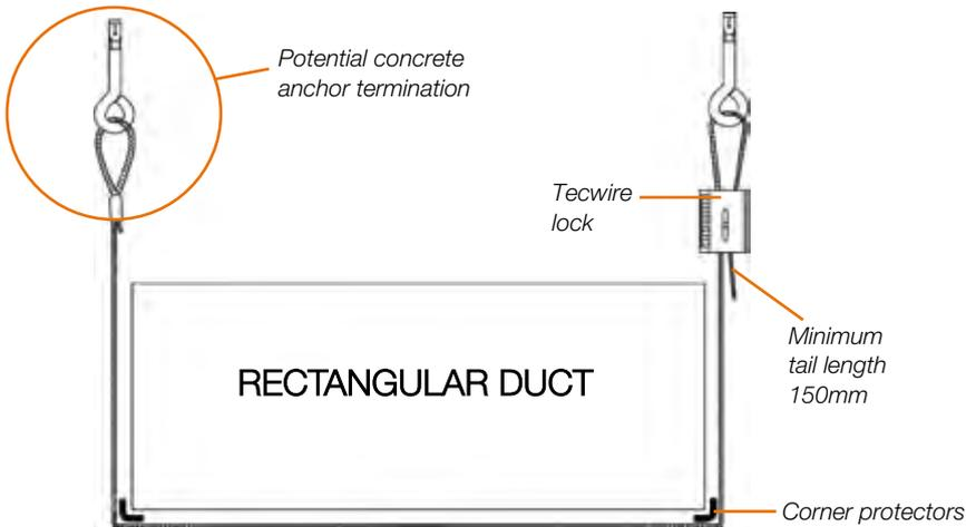
To support rectangular ductwork using the cradle method, there are a range of termination options to suit various substrates and steelwork:
