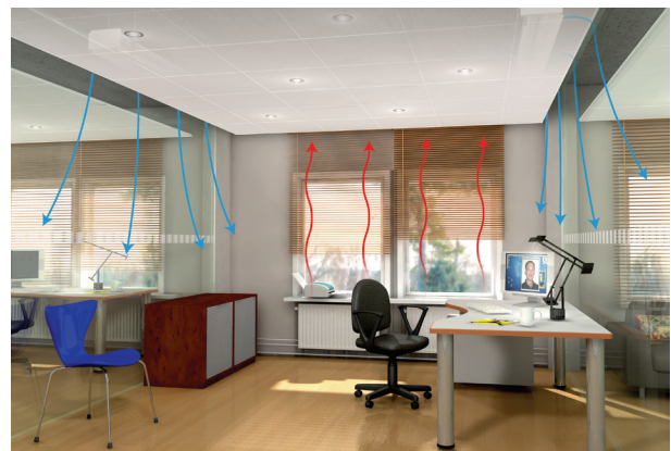
Picture 2. Celo's technical solution is based on a unique technology, patent applied for, where the cooled air is carried down through an outlet slit in the suspended ceiling, then along the wall and down towards the floor.
